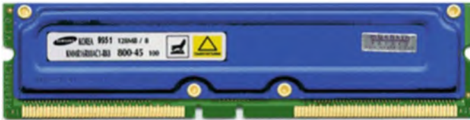
Fig. 7.5 Rambus memory module (Courtesy Samsung Corp.)
