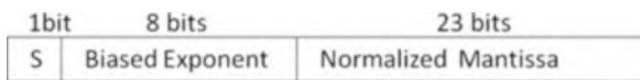
Fig. 1.10 IEEE 745 floating point single precision (S = represent sign of mantissa. S = 0 means mantissa is positive, and S = 1 means mantissa is negative)
